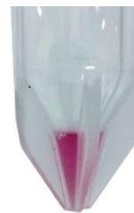
Figure 3: Example of 500 \mu L in the GELATION TUBE (DMEM is used for instruction purpose)
