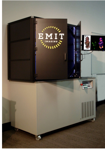
Figure 1: Cryo Fluorescence Tomography System comprised of an imaging chamber on top of a cryo sectioning system. Optical magnification allows the system to vary the FOV and resolution.
